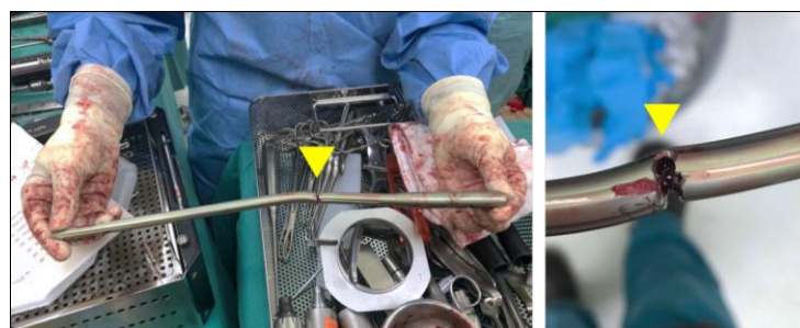
Fig 4: Intraoperative photographs. Left: Removed bent intramedullary nail. Right: Close-up view of burred site of bent intramedullary nail. Yellow Arrow points to the site of burring in both photos.
